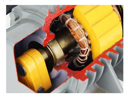
Cleveland Vibrator maintains its own repair department, staffed by experienced and quality personnel. Reconditioning of rotary electric vibrators involves rewinding, dipping and baking the stator, reinsulating the windings, and replacing bearings, power cord, leads power terminal block, etc. The cost of reconditioning generally runs approximately 50%-60% of the cost of a new unit and is covered by the same warranty, if the unit was originally purchased from Cleveland Vibrator.
