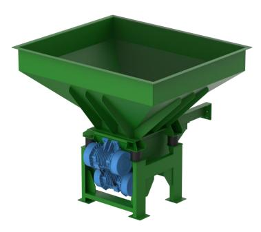
Rotary Electric Vibrators positioned on a volumetric vibratory feeder.
